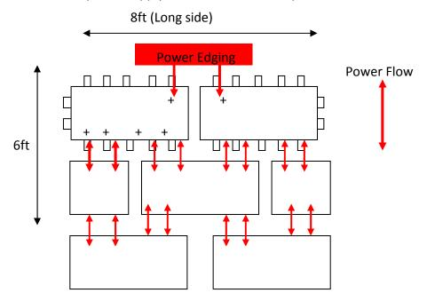
Regardless of most sizes, this power flow principle applies. This system therefore ensures that power flows to all the floor panels even if one panel is not receiving the power as it should for some reason (See trouble shooting guide if you are experiencing trouble with your floor)
