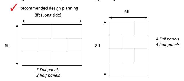
By designing the floor the long-side first, you use less half panels yet the floor is the same size 24ft<sup>2</sup>.
