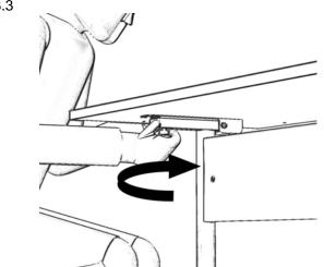
Tighten the handwheel at either end of the baseframe to secure the top
