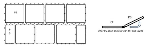
! The five top LUGS on the panels used in the second and all following rows are designed to slide under the rim of the frame on the adjacent panel. Holding the panel at an angle of between 30° and 45°, slide the lugs under the panel above. When the two panel frames are touching along the whole length of the panel, gently lower the panel into place.
