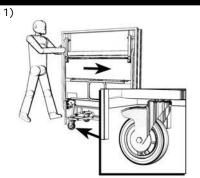
Wheel into position & lock castors. Push only from the steering end.
