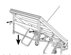
Remove the two pins from the telescopic leg, extend the leg until the next set of holes align, then replace the two pins. Repeat on other side.
