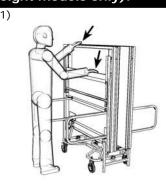
Hold first half as shown & pull on leg to unlock.
