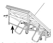
Remove the two pins from the telescopic leg, push the leg up until the holes align, then replace the two pins. Repeat on the other side.
