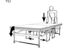
Push down on one end to set the platform on the ground. Ensure the second-height legs are fully open.
