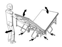
Lift the platform half and pull backwards to rock the base frame to the ground. Ensure the base frame and all four fold out legs are in contact with the ground.
