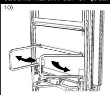
Release the Velcro straps and fold out the second-height legs on both sides of the platform.
