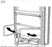
Fold away the second height legs and secure the Velcro straps.
