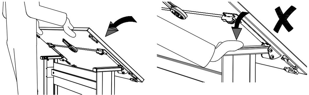
2.3.3 Push down on the top to ensure both latches have engaged.
