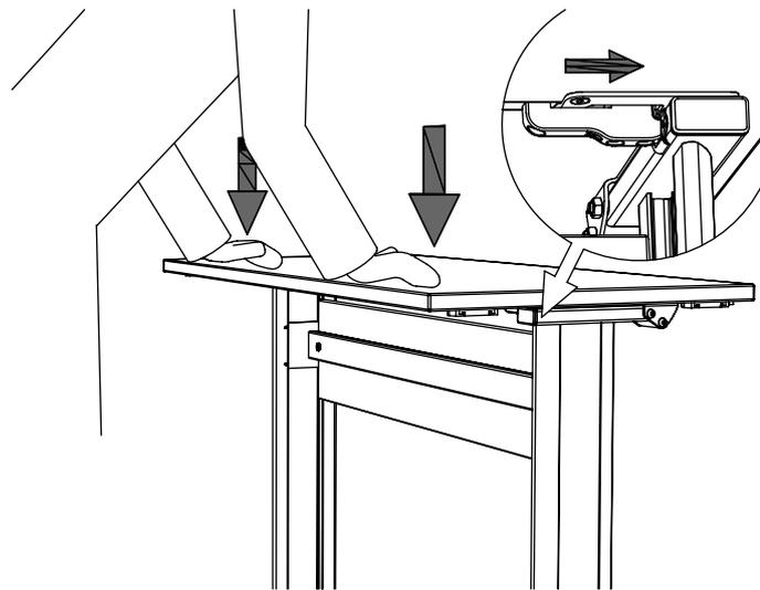
2.3.4 To release the top, operate the release handle by turning in either direction, then lift the top to its upright position.
